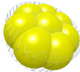
Fig. 6. Shape of biconvex tablets according to the glued-spheres approach
