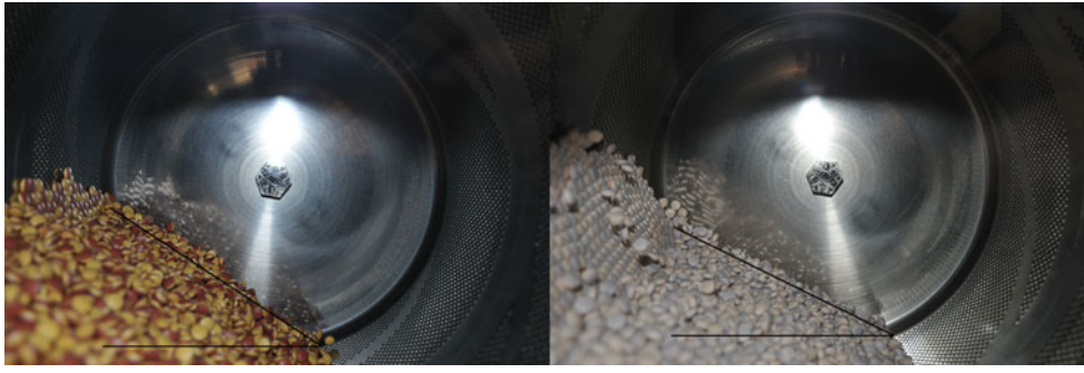
Fig. 5. Moving tablet bed of GITS ( left ) and active-coated GITS ( right ) at 16 rpm drum rotation speed
